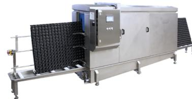
As part of our drying options, we can offer you centrifugal drying systems. In three options, horizontal -, vertical – and stack centrifuge. This type of drying is extremely energy efficient, compared to conventional drying while the rotating drum is driven by an electric motor and due to the centrifugal force, the washing water is flung off the products
