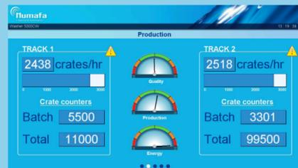
Numafa offers a Management Information System with its machines. With this system, the operator can easily monitor the desired parameters for your (washing) process and gives tools for guidance.
