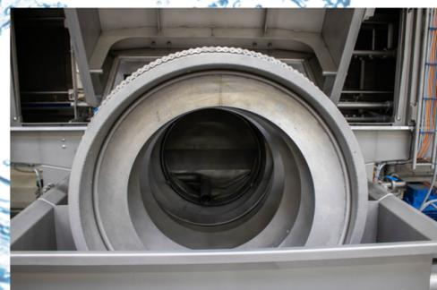
The High Pressure Label Remover (HPLR) removes different kinds of labels that are placed on the crate during its cycle in the supply chain. To make sure all kinds of labels are removed, Numafa used different configurations of pressure and nozzles within the HPLR.
