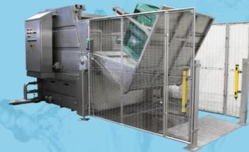
The Numafa container washer line ranges from the cleaning of 200 liter standard carts to 1000 liter containers. With a range of cleaning 25 to 300 containers per hour.
