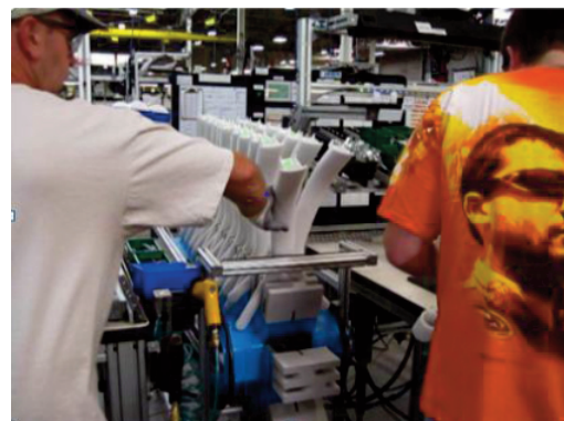
The returnable packaging “self-returns” so the operator assembling the chair doesn't have to stop what he is doing to return the packaging.
